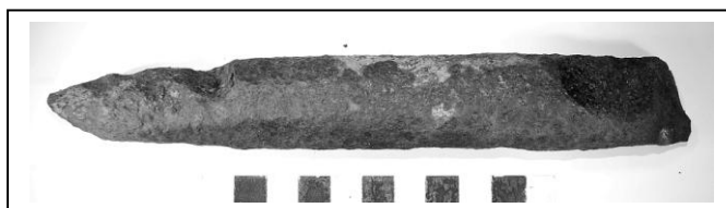
Fig. 9 Tapering steel with a round ground tip and broken opposite end. It may represent the broken pick point of a poll-pick – used by miners to knock wooden props into place. # DWA209IR/F10//MO6.
